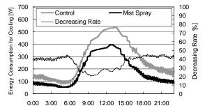
Figure 11: Comparison of Variation with Time of the Electricity Consumption Reduction for Cooling by Use of Mist Water Spray to the Outdoor Unit of Air Conditioner (September 22)
