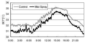
Figure 10: Comparison of Variation with Time of SET\* by Use of the Mist Water Spray at Balcony (August 16)
