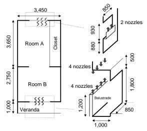
Figure 6: Details of the nozzle setting for the veranda spraying test
