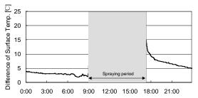
Figure 9: Variation with Time of Surface Temp. Reduction by Use of the Mist Water Spray at Rooftop (August 16)
